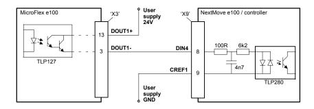
Figure 33 - DOUT1 - typical connections to a Baldor NextMove e100
